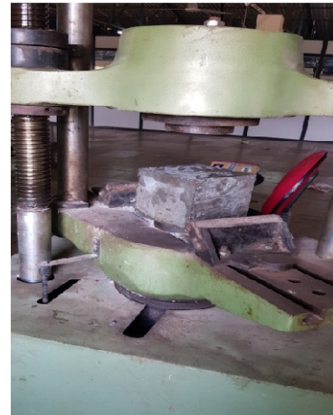
Figure:-13 compressive strength test as per IS 456-2000
