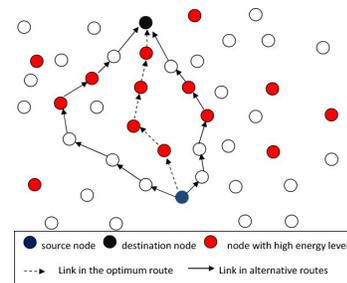
Fig. 1 Optimum route selection in FF-AOMDV
