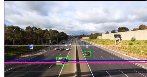
Fig. 4 Detected Vehicle. Output of background subtraction, Erosion, Dialation, Detected bounded box
