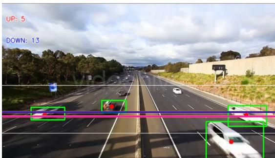
Fig. 5 Vehicle Counting (up and down)
