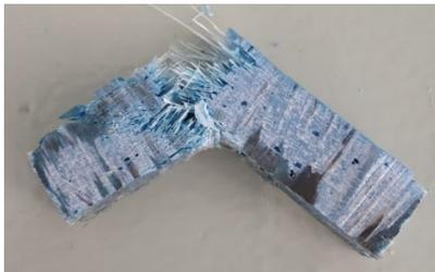
Fig. 5 Hardness test sample
