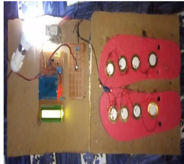
Figure 7: Prototype of Piezoelectric Footstep Power Generation
