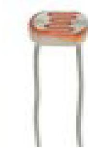
Since we want to be able to track the sun we need some form of light detector. There are a number of alternatives here, but the simplest is an LDR (Light detecting diode)
