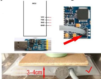
Fig.2 the pressure sensors module experiment platform
