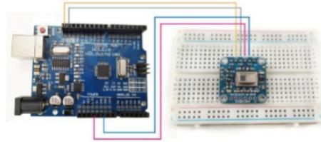
Fig.3 the infrared imaging sensor experiment platform
