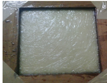
Fig 3.4 Hand Layup Process
