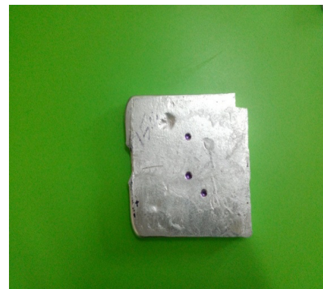
Fig 3.5 Specimen – III (AA7075 95%, WC 3%, SiC 2%)
