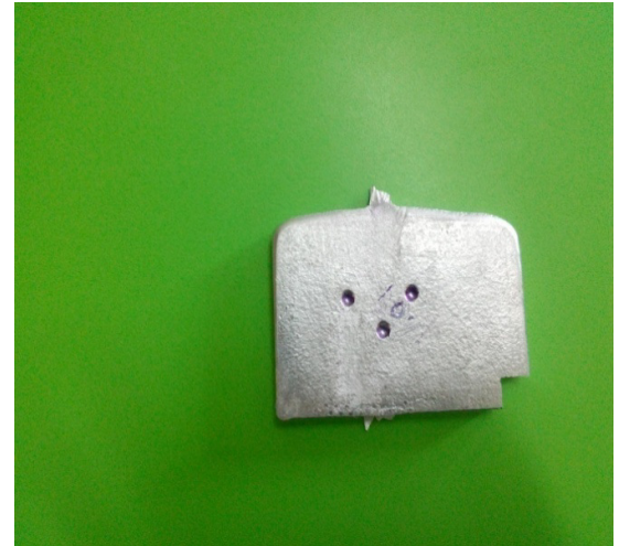
Fig 3.4 Specimen – II (AA7075 95%, WC 2%, SiC 3%)
