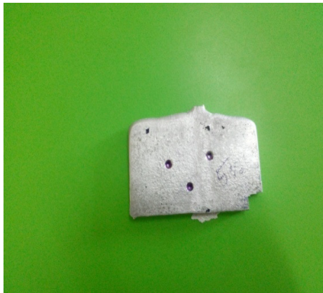
Fig 3.3 Specimen - I (AA7075 94%, WC 3%, SiC 3%)
