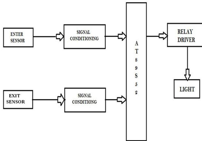
The basic block diagram of the bidirectional visitor counter with automatic light controller is shown in the above figure. Mainly this block diagram consists of the following essential blocks.
